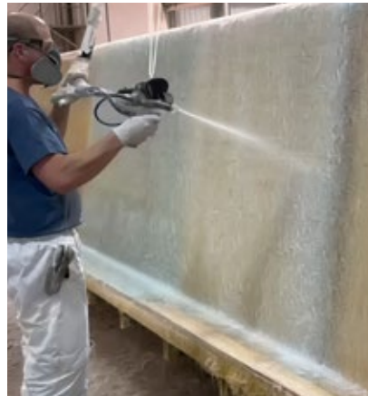
5 Simultaneous Resin & Fiber Spray
